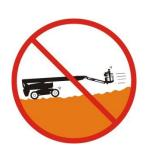
Reduce the transfer speed according to the conditions of the ground, the traffic, the slopes, presence of workers or other factors which can cause collisions.
