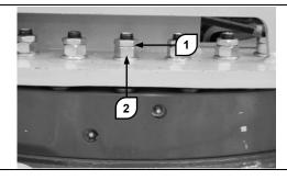
Check the turret fixing nuts on the slewing ring gear. Check for rusted, slackened or missing nuts.
