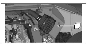
2 Release the catches and remove the cover on the front of the filter.
