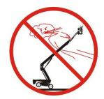
Use utmost caution and low speed when the machine is moved with the platform retracted on surfaces that are irregular, unstable, with detritus or slippery, or near ditches and cliffs.
