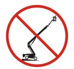
Do not raise or extend the boom unless the machine is placed on a stable level surface.
