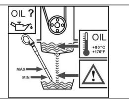
An insufficient and/or excessive lubricant oil level can damage the engine. Check the oil level only with the engine horizontal and stopped. Check the lubricant oil level only while it is warm, 5 minutes after the engine is switched off. Do not remove the oil level rod with the engine running. Danger of burns.
