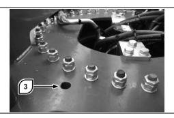
To check the fixing screws of the slewing ring gear on the chassis, align hole 3 with the screw underneath by rotating the turret.
