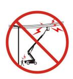
Move away from the machine in case of contact with live electricity lines. Workers on the ground or on the platform must not touch or operate the machine until the electric power supply has been disconnected.
