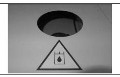
Note: The hydraulic oil should be applied to the local environment, and be filtered at the accuracy of 20  $\mu$  m.
