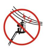
Observe the local and national regulatory standards in force concerning the distance required from electricity lines. At least the safety distance indicated in the Table below must be respected.
