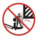
Take extreme care while gripping the platform railing to prevent danger of crushing.
