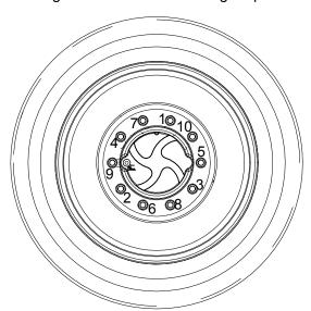
When there is sound like 'kada', the lug nut is fastened at proper torque.
