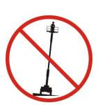
Never exceed the maximum permitted inclination of the truck; the maximum permitted inclination of the truck is indicated in the technical specifications and on the ID plate on-board the machine.
