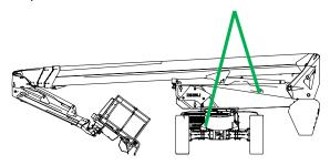
Adjust the lifting devices in such a way as to keep the machine level and without causing damage to it.
