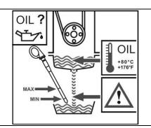
An insufficient and/or excessive lubricant oil level can damage the engine. Check the oil level only with the engine horizontal and stopped. Check the lubricant oil level only while it is warm, 5 minutes after the engine is switched off. Do not remove the oil level rod with the engine running. Danger of burns.
