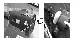
3 Grip the filter element and remove it from its seat.
