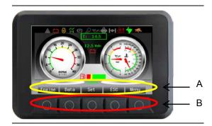
This panel contains the basic information for monitoring the working of the truck. The pages and options available are displayed in the lower part of the screen [A] and are controlled by the corresponding buttons present below [B].
