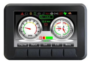
The setting interface could be entered by depressing setting button and hold on for one second. The optional function can be turned on or off without password, after entering setting interface. The procedures are as follows:
