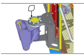
Check if there is some bolts is slacken or missing and the sensor undamaged. If there is abnormal condition, ask for help from DingLi or your agency.
