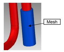
4 Clean the mesh slightly. The corrosive chemical solvent should be forbidden to use.
